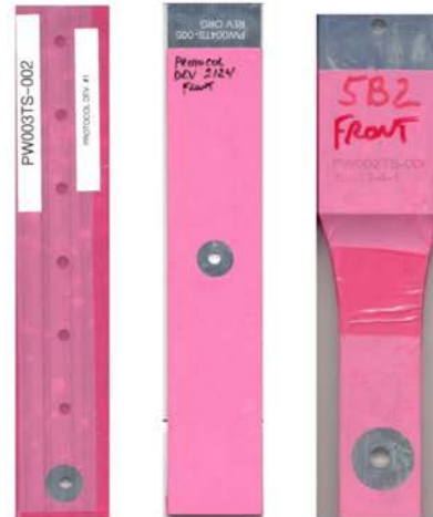
Figure 6 (L) Representative image of a multihole protocol development specimen taped off to expose one bore hole for corrosion testing; (C) Representative image of a single hole protocol development specimen taped off to expose one bore hole for corrosion testing; (R) Representative image of a dog bone fatigue test specimen taped off to expose the bore hole for corrosion testing (note: only top 2/3 of dog bone visible in scan image, although entire dog bone was taped).
