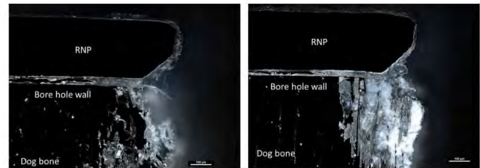
Figure 24. Dark field image of RNP-sealant/bore hole wall interface on back of dog bone. (Left) Orientation "A". (Right) Orientation "B".
