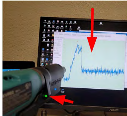
Process Control Software Identifying Successful Installation
