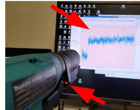
Process Control Software Identifying Unsuccessful Installation with LED and Red Graph
